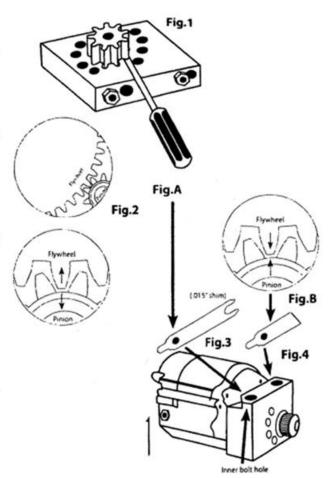
**NOTE:** Check the starter end plate is correctly mounted and fasteners are tight to avoid any pinion gear / drive mesh problems.
