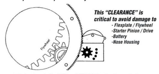
This is not needed for FORD and CHRYSLER as they have a fixed starter pinion to Flexplate / Drive plate clearance.
