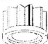
Incorrect Wear Pattern Too Much Clearance (Use Less Shims)
