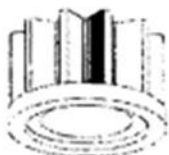
Incorrect Wear Pattern Not Enough Clearance (Shims Needed)
