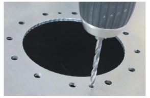
8. Using a 4mm drill bit, drill through the fuel cell on both marked holes.
