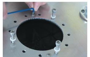
**12.** Tighten the bolts using a 2.5mm Allen key. Use three of the bolts from the head unit to align the c-ring correctly.
