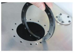
**10.** Insert the C-ring as shown using the cut-out in the ring to fit through the hole cut-out in the top of the fuel cell.
