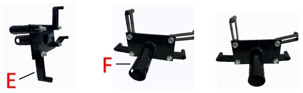
7. Once the Mounting Arms are attached you can now slide the whole Mounting Plate (F) into the main frame (A). Use the Locking Pin (I) to secure the Mounting Plate. Insert the Handle (K) in the back of the Mounting Plate. To rotate the Mounting Plate, you will have to lift the Locking Pin out and rotate with the Handle then insert the Locking Pin back in to secure the Mounting Plate.
